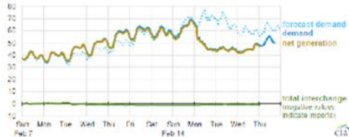
Hourly electricity demand, net generation, and total interchange (Feb 7–Feb 16, 2021) Electric Reliability Council of Texas, Inc (ERCOT) gigawatts
