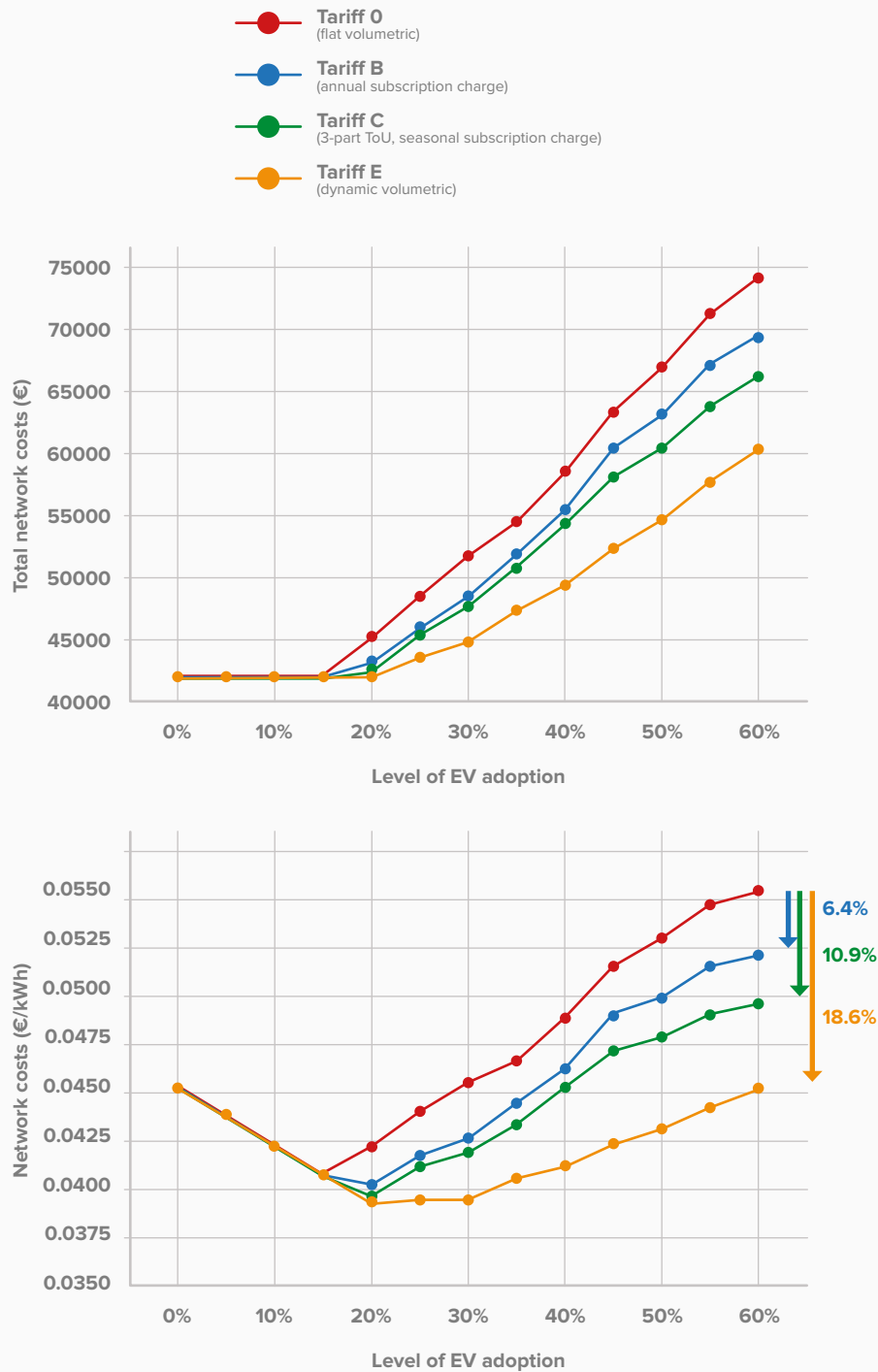
FIGURE 4.4 — Total network costs (€) and network costs (€/kWh) under each modelled tariff design
